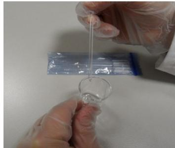
For samples in liquid form such as GHB, we advise to use the round end of the supplied spatula or otherwise use a pipette and insert one (1) drop into the ampoule.
