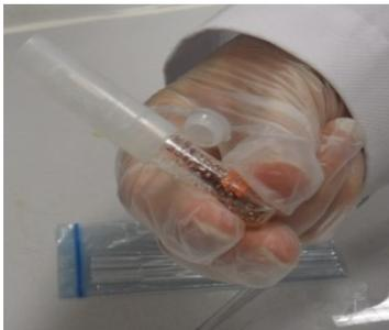
Compare the color from the reagent granulate with the color line printed on the ampoule or as printed on the pack.
